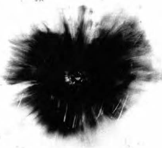
FIGURE 28 Bullet Hole In Polyethylene Sheet
