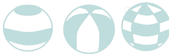
Figure 2.4: Graphical views from the side of objects. The left and right pictures represent the zonal and tesseral harmonics respectively while the middle one represents sectorial harmonics.
