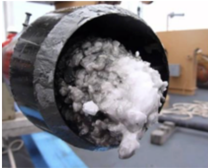
Figure 2. The growth of gas hydrates in an oil pipeline. (Image by Bill Schmoker, PolarTREC).
