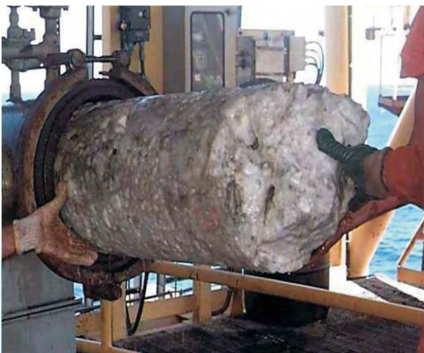
Figure 2: Image of a methane hydrate buildup in an oil pipe
