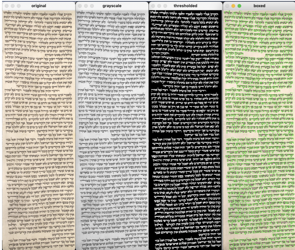
Figure 4. The four stages necessary for preprocessing and segmenting an image (ibid)
