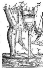
Figure 4: Pare's drawing of his prosthetic leg design [24]
