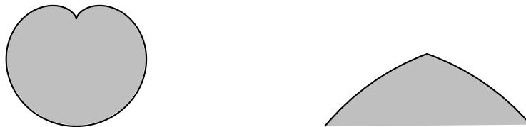
FIGURE 1. A scatterer with a convex corner point (left) and a concave corner point (right)
