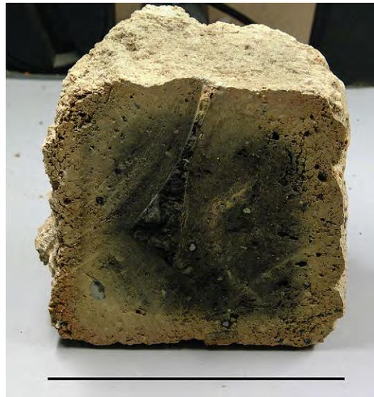
**Fig. 8.** Section of one of the bricks from wall 123007 showing that the brick was exposed uniformly to heat on all surfaces.
